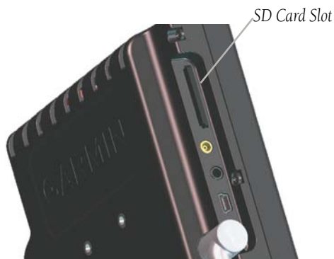
GPSMAP 695/696 SD Card Slot
